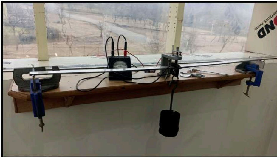
Experiment to measure the Young's Modulus of steel
