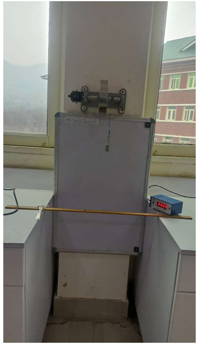
Flywheel to measure moment of inertia
