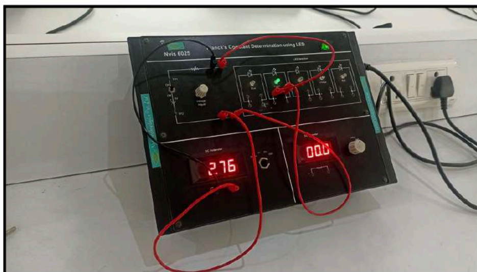
Experiment to measure the value of Plank's constant
